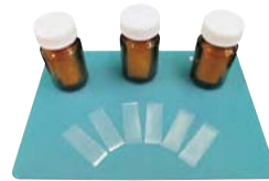
Standard Samples Containing Phthalate Ester for Py-GC/MS
